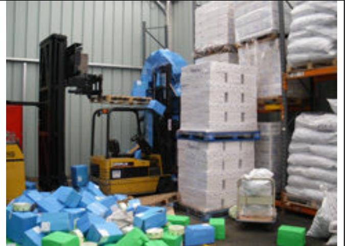
The HSE investigated the incident and found the racking was in a poor condition. The rack's horizontal beams were not properly engaged in the uprights and hadn't been secured with locking pins. The company was issued a Prohibition Notice, which ordered workers to stay out of the warehouse until the racking was made safe.
