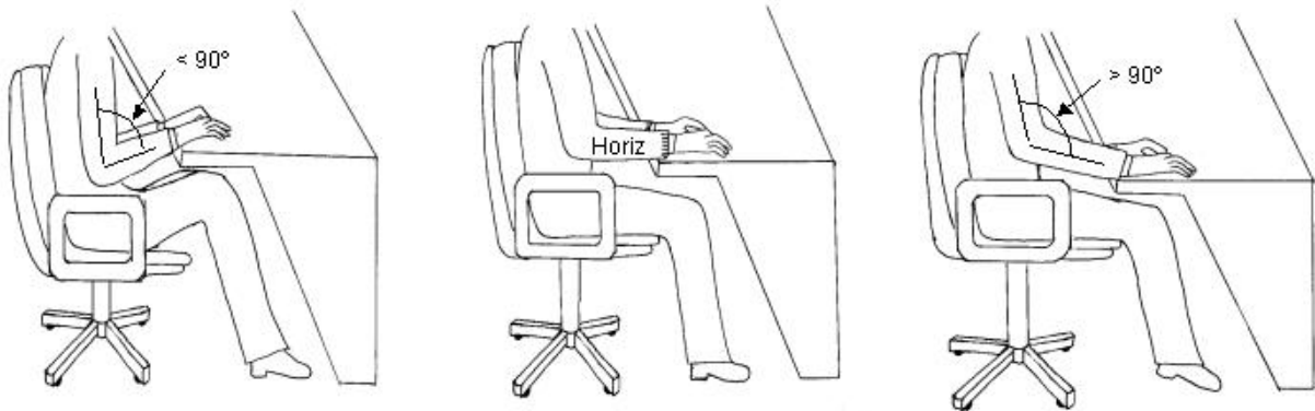
Fig. 3 Effects of correct and incorrect seat heights
