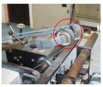
This is a terrible example, showing how maintenance crews were ignorant about the function of the immediate guard. Note that, probably following a beltbreak, they have positioned the guards on the *outside* of the belt, rather than the inside.
