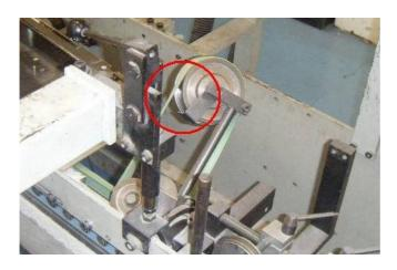
This is an example of a poor immediate guard. It is obvious that it has slipped as in B above, but even if it were properly adjusted, it would create a wedge as in C above.
